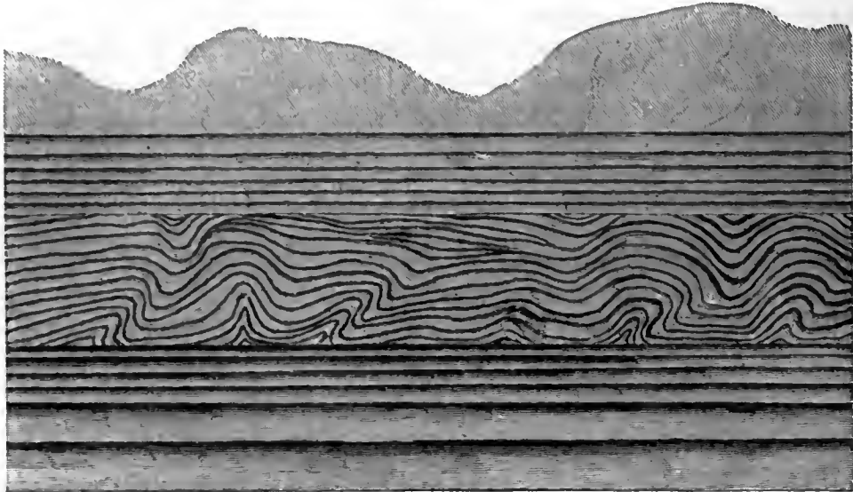
Section on the feeder of Black river, showing local movement in a portion of a series of thin clay beds or layers, those above and below being wholly unaffected by the movement which deranged them. This shows the least amount of disturbance of any of the three sections.
